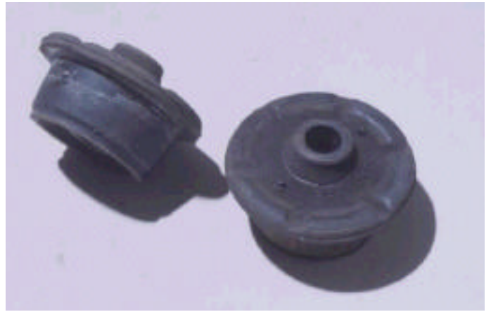
The original tie bar bushes
