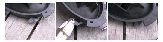
**5.**) Re-trim the hole through which the pull cable passes. File off.
