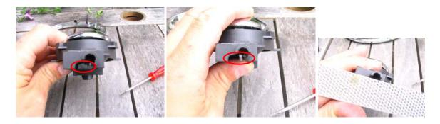
**6.)** Prise out the plastic circlips that held the old cable.
