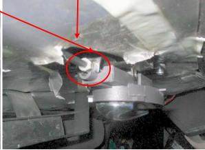
**14.)** If you remove the doorpanel. Do not take the <u>door card</u> separately from the door panel. Let it in one whole assy. Easy for trial fitments. Easy on/off. You might need to trim down the cardboard (1) from the door panel. And possibly(?) the metal flanges (2).
