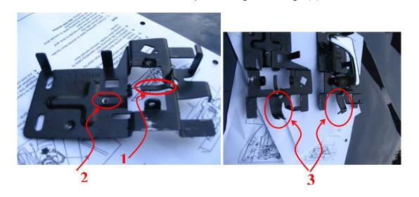
8.) Loosen the screw of the OEM MGF bracket and prise out the cable. If you have the opportunity, shorten the cable by ½" (1,25cm). I didn't and there's some slack in the R75 handle when fitted. First check what you need in order to do this and to remount the end of the cable that fits the R75 hinge!!
