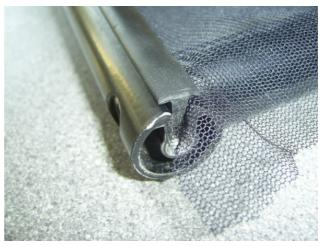
7. When you have put the bottom rubber into the recess and given it a sound tap (a rubber mallet was useful here) start from one side of the frame and stretch the fabric whilst inserting the rubber over it and into the groove. Don't worry if you do a bit and it looks ruffled, just go back and try again.
