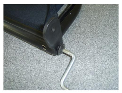
These are held in place by one screw either end of the wind stop. Use a 4mm allen key to remove them and pull out from the tube.
