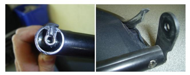
The mesh is held in by two rubber strips that push it into a recess around the top and base of the tubular wind stop (as in the left hand photo). Gently remove the rubbers and set aside.
